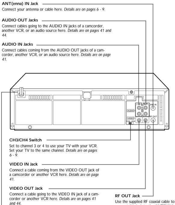
connect this jack to the ANTENNA IN Jack on your TV or to the IN Jack on your Cable Box/DBS (if applicable). Details are on pages 6 - 9.
